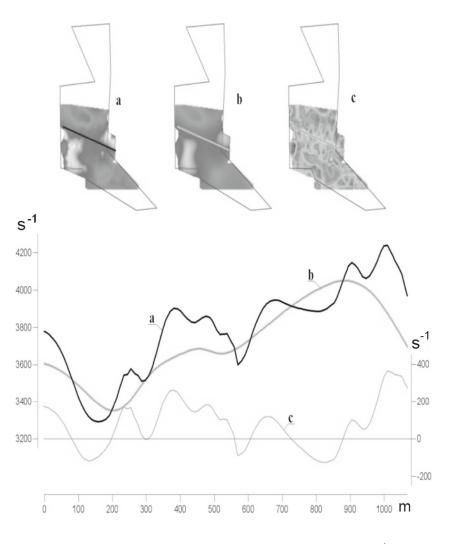
**Fig. 3** Diagram of original (**a**), averaged (**b**) and the local component (**c**, c = a-b) of the field of gamma radiation in the "Red Forest" area. At the top is the position of the line of graphs on the respective maps be up to 2 m; the trench depth is about 2 m. Currently trenches and piles are practically inconspicuous because of the subsidence of the soil and thick vegetation cover.
